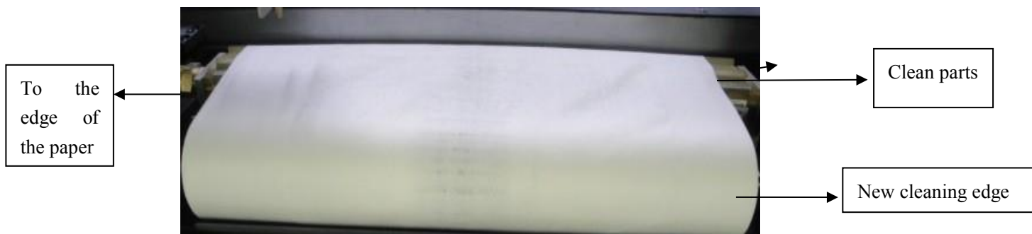
Figure 7-2 Cleaning paper installation
