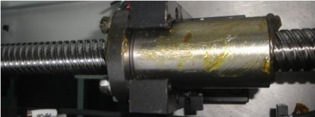
Figure 7-17 Cleaning and lubrication of screw rod and guide rail.
